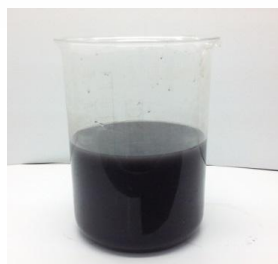
Figure 1. The wastewater from the washing flexography printing machine does not precipitate.
