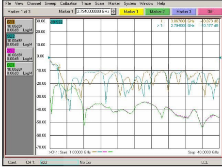
Fig.3 The measured reflection coefficient ( S_{11}, S_{22} ) and the transmission coefficient ( S_{21}, S_{12} ).
