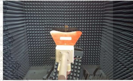
Fig.5 Measurement set up in Reflection coefficient and pattern.
