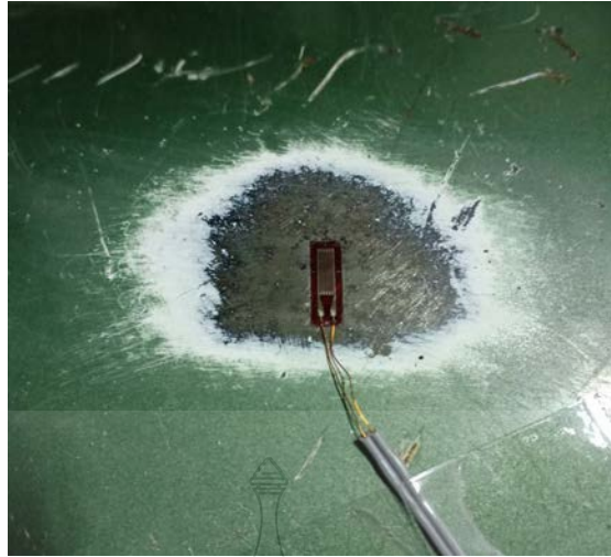
Figure 6 The installation of the FLA-6-11-1L type strain gauge sensor on the pressure vessel.
