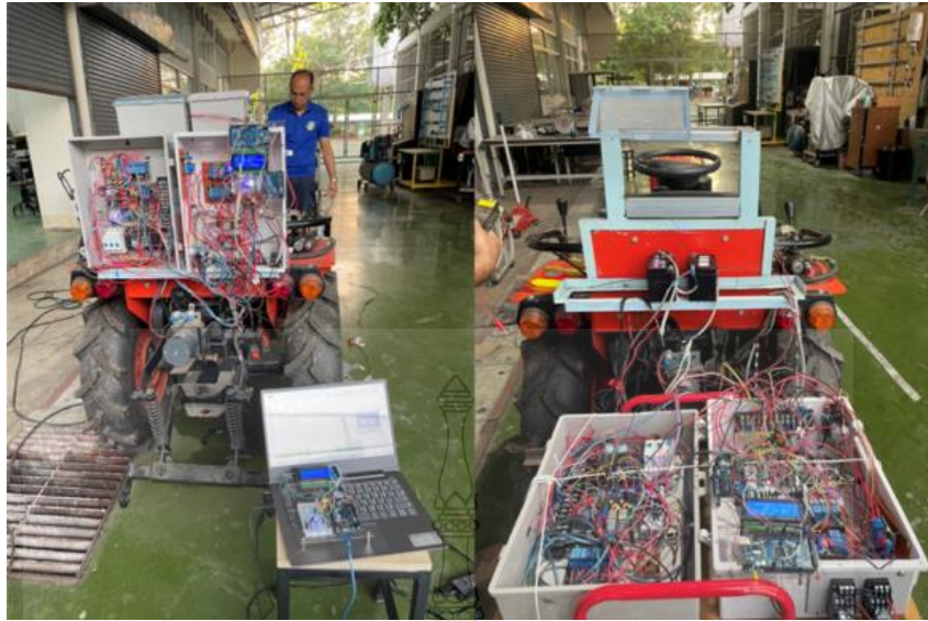
Figure 4.51 Separating The Control Box From The Tractor Body
