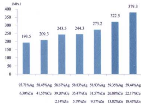
Figure 2 The graph representing the tensile force of the alloy specimen (MPa)
